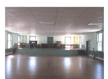
Second floor: Stage at south end of the Assembly Room. The rear window was blocked in when the stage was installed. The egress door at right was converted from a window when the fire escape was installed.
